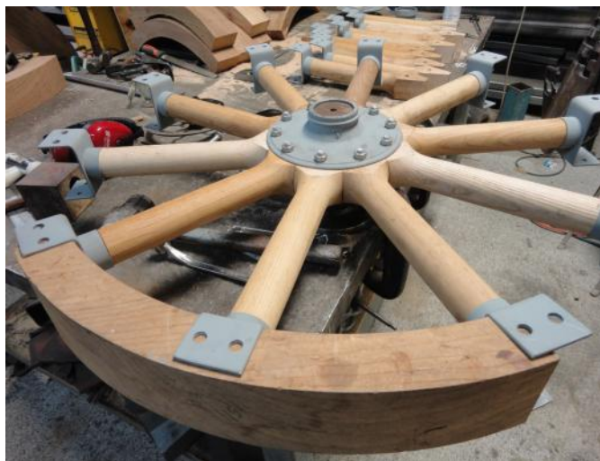
Spokes shortened & turned to receive felloe sockets.
