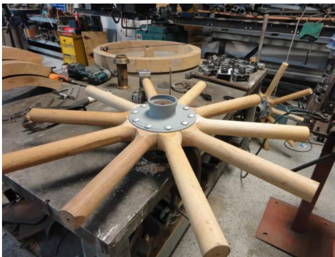
Spokes fitted to flanges with bolt domes machined.
