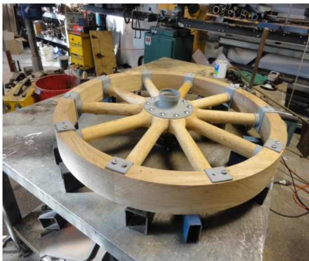
Felloes fitted, & dressed to correct size awaiting tire. (tire size 90mm x 10mm x 880mm diameter) (holding Tec screws temporary)
