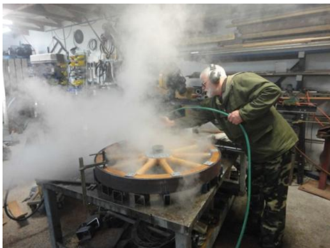
Roy Parker with hose cooling tire, a cloud of smoke & steam ensues. (how to fix a cold fast)
