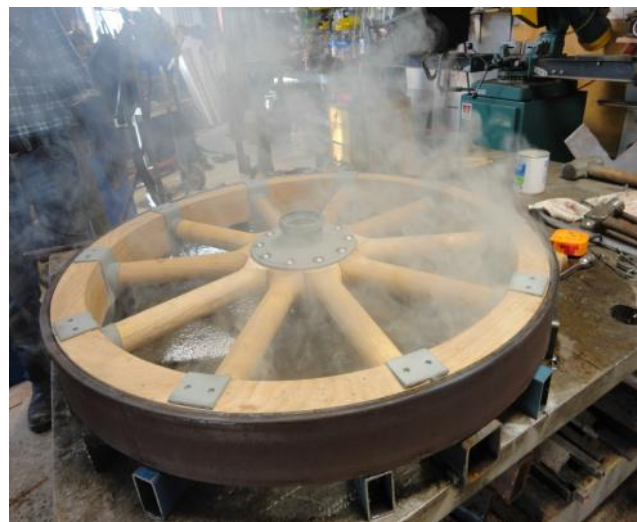
Tire heated to size now dropped over felloes in moments before shrinkage contact smoke up
