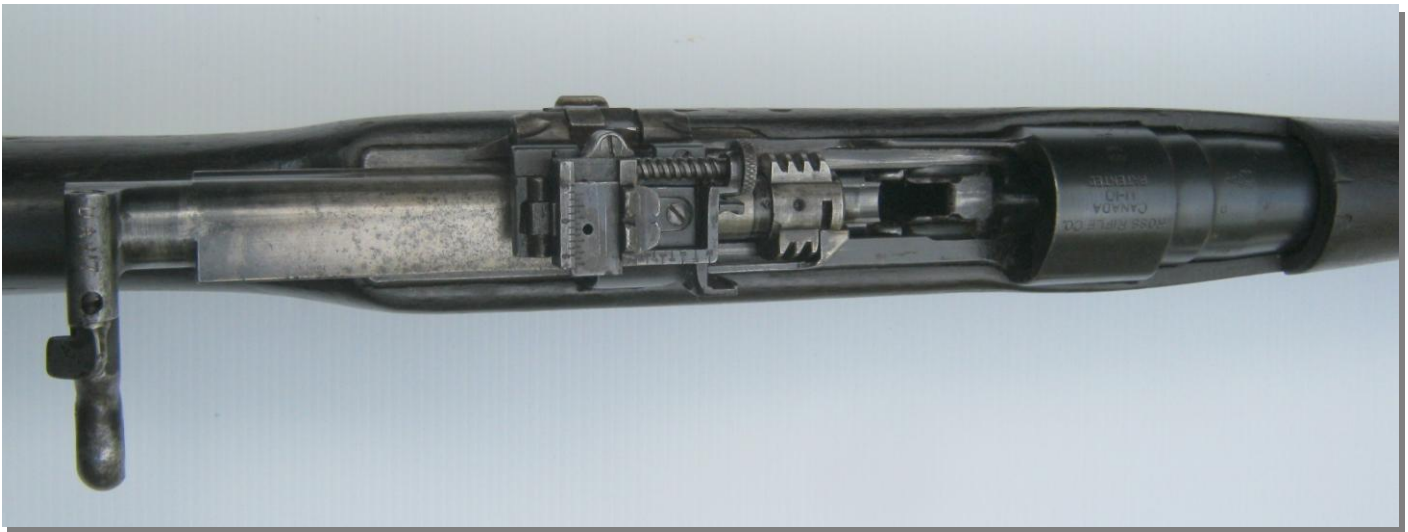
Straight pull bolt withdrawn to the rear, note screw thread locking lugs
