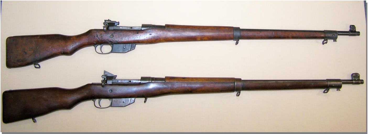
The Mk IIIB British contract (bottom) is similar but has different sights which are similar to the P 14.
